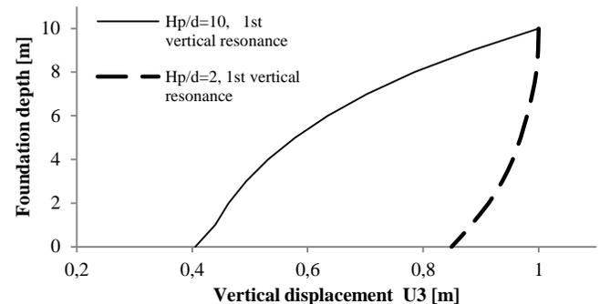
Fig. 9: Distribution of the foundation vertical displacement along the depth at the 1<sup>st</sup> vertical eigenfrequency of the soil layer for the case 1 and 6.
