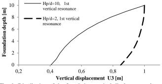
Fig. 9: Distribution of the foundation vertical displacement along the depth at the 1<sup>st</sup> vertical eigenfrequency of the soil layer for the case 1 and 6.
