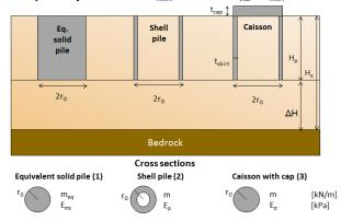
Fig. 4 Foundation geometries investigated for the case of caissons.
