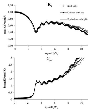
Fig. 7: Variation of the vertical dynamic stiffness and damping coefficients with respect to the non-dimensional frequency. Effect of the foundation geometry on the real component and the imaginary component for case 6.
