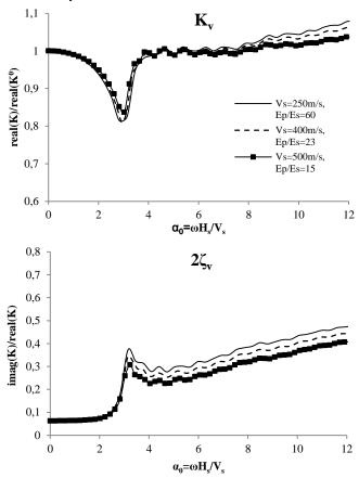
Fig. 6: Variation of the vertical dynamic stiffness and damping coefficients with respect to the non-dimensional frequency. Effect of the stiffness of the soil layer on the real component and the imaginary component for cases 1, 4 and 5.
