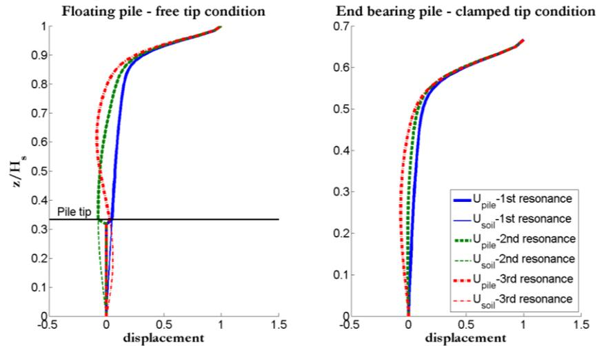
Figure 3. Distribution of the soil and pile displacement along the normalized depth  $z/H_s$  at the three first eigenfrequencies of the soil layer. The floating pile (a) and the end bearing pile (b) for the reference case are shown.
